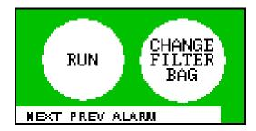
"Run/Filter Warning" will display when the pump is running
