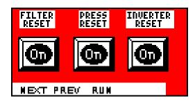
"Filter Reset". In the event a clogged filter bag significantly impedes the flow of coolant, the pump will activate an E-Stop condition and the "Filter Reset" light will go on. The filter <u>must</u> be changed at this time. When the bag is changed the filter reset must be pushed to clear the alarm.
